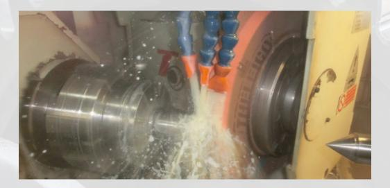
Synthetics are oil free cooling lubricants. They consist exclusively of water soluble components which provides three essential distinguishing features compared to emulsions:
